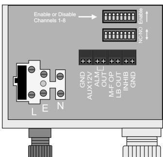
Figure 5. Enabling & Disabling Inputs/Channels
