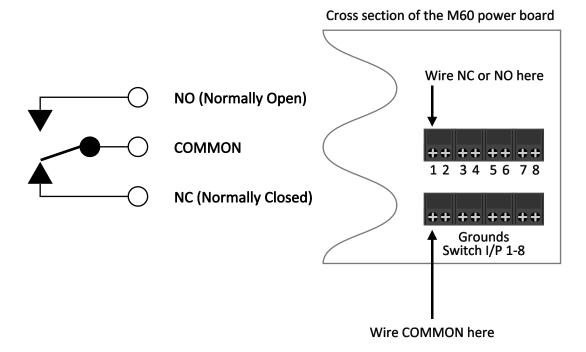
Remember you must set the appropriate DIL switch for each of the M60 inputs, to either Normally open (NO) or Normally Closed (NC), depending upon the input type connected.
